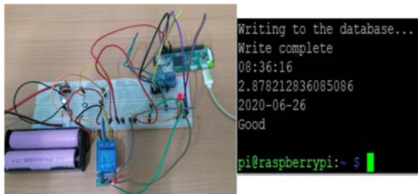
Fig. 12. Initial setup for fault detection.
