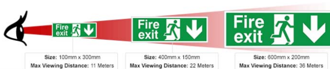
Fig. 1: Exit signage visibility.
